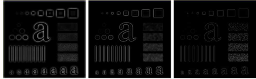
FIGURE 4.55 Results of highpass filtering the image in Fig. 4.41(a) using a BHPF of order 2 with D_0 = 30, 60, and 160, corresponding to the circles in Fig. 4.41(b). These results are much smoother than those obtained with an IHPF.
