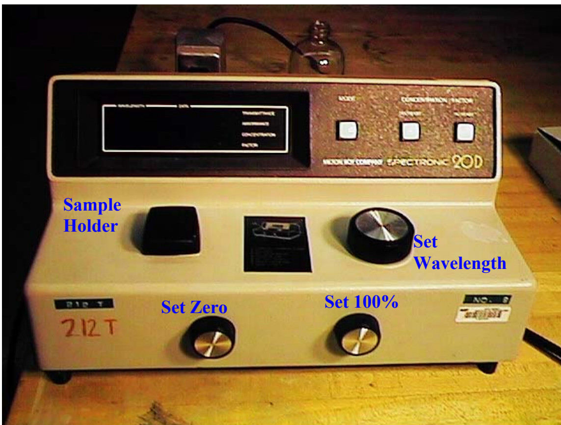
Figure 2. Apparatus for the determination of the transmission and absorbance of a sample, a spectrophotometer.
