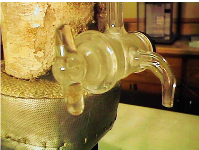
Figure 2. Three way stopcock for Cottrell boiling point apparatus.
